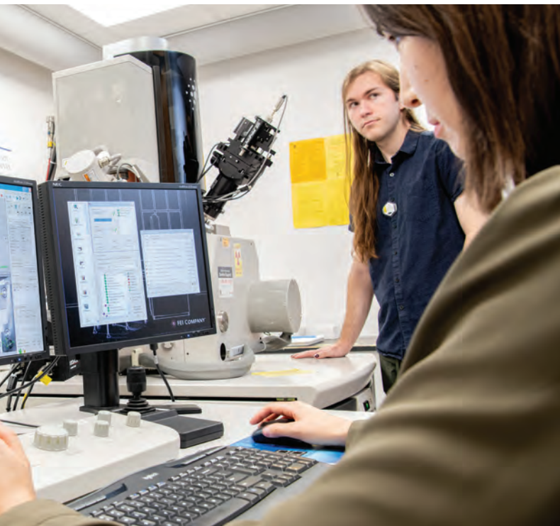
Left: Assel Aitkaliyeva with a transmission electron microscope. Above: Operating a focused ion beam instrument with doctoral student Jack Mayer. The specialized tools enable her group to prepare and study samples of nuclear material to better understand their structure and origins.
